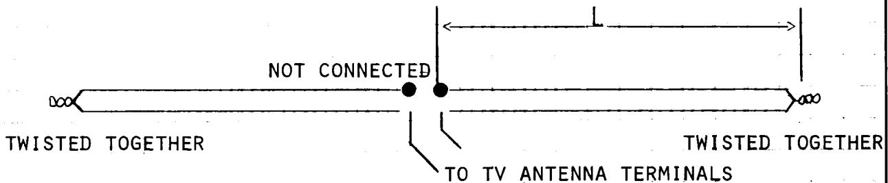
Use ordinary lead-in (flat) wire. Twist wire together as indicated above after cutting as shown. Connect to TV set antenna terminals. Adjust direction of the antenna for the best picture. Leave gap at the top, as shown. Tape bare wires.
