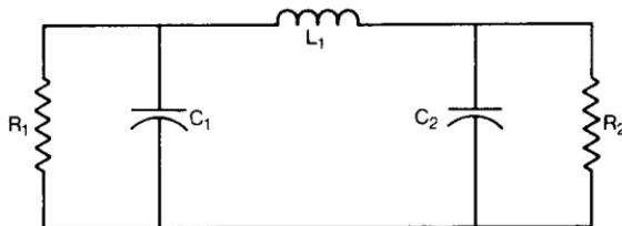
Given the values of  $R_1$  and  $R_2$ , the frequency ( $f$ ), and the desired circuit  $Q$  (center frequency/desired half-power bandwidth), the values of  $C_1$ ,  $C_2$ , and  $L_1$  are found from the following formulas.
