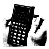
When the motor stops, remove the card from the left side of the calculator and insert it in the upper "window slot" on the right side of the calculator.
