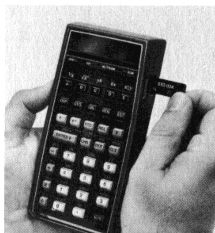
When the motor stops, remove the card from the left side of the calculator and insert it in the upper "window slot" on the right side of the calculator.
