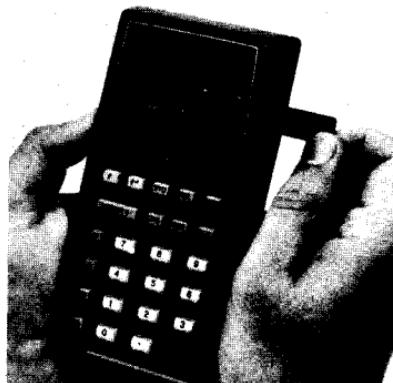
When the motor stops, remove the card from the left side of the calculator and insert it in the upper "window slot" on the right side of the calculator.
