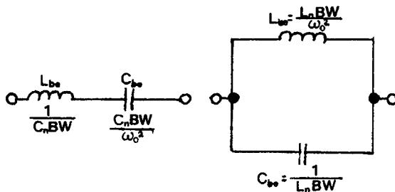
A bit of thought may be necessary to determine whether the L-C's are connected in series or parallel.
