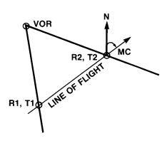
The distance from the VOR station to the aircraft at time T2 is given by
