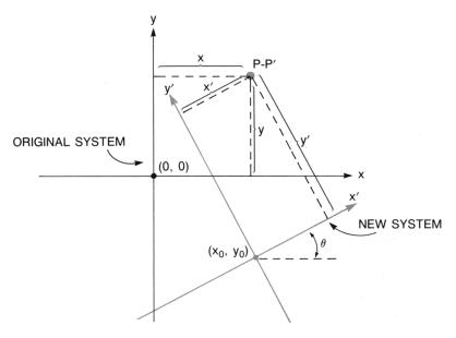
After specifying the new origin (x, y, z), you specify the rotation angle. For a three-dimensional system with a non-zero angle of rotation, you also specify its *rotation vector* (a, b, c). The rotation vector defines the axis about which the rotation is to be done; it can have any non-zero magnitude.
