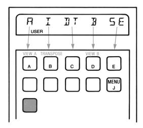
This menu shows you the choice of matrix operations you have in MATRX. Press J to recall this menu to the display at any time. This will not disturb the program in any way.
