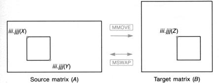
When an input of the form iii.jjj is expected in the X-register, a zero value for either the i-part or the j-part is interpreted as 1. (Zero alone equals 1.001.) This is true for the iii.jij-values that MMOVE and MSWAP expect in the X- and Z-registers, but not for the pointer value in the Y-register.
