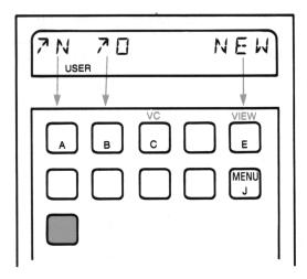
Once you have entered your variables, this menu shows you which key corresponds to which function in TR. To restore this menu to the display at any time, press J if the USER annunciator is on. (If it is not on, press USER to turn it on.) Or, if the calculator is displaying results, you can press [R/S] until the menu appears. This will not disturb the program in any way.
