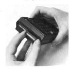
Plug in any additional application modules, also after the last memory module. Cover any unused ports.
