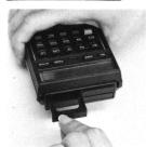
In an HP-41C, insert the application module into any port *after* the last memory module. (HP-41CV's and HP-41CX's don't use memory modules.) Insert the module with its label right-side up, as shown. For example, if you have a memory module in port 1, you can insert an application module into port 2, 3, or 4. (The port numbers are diagrammed on the upper back of the calculator.) *Never insert an application module into a port with a smaller number than a memory module's port.*
