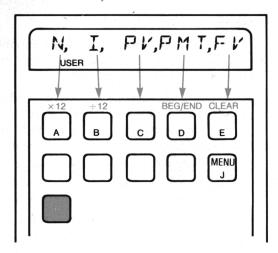
This menu will show you which key corresponds to which function in TVM. Press J to recall this menu to the display at any time. This will not disturb the program in any way.
