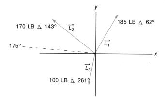
Save the results for the polar coordinates of  $L_3$  and the 175°-line so that you can re-use them to find the resolution (dot product) when  $L_3$  is doubled. This example stores those results in vector-registers 1 and 2. This solution uses Alpha (manual) execution of the vector operations, but you can use the Vector Calculator, as in the above example. Make sure that the User keyboard is not active.
