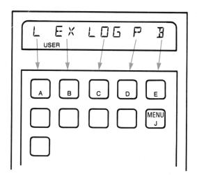
To clear the menu at any time, press •. This shows you the contents of the X-register, but does not end the program. You can perform calculations, then recall the home menu by pressing J. (However, you do not need to clear the program's display before performing calculations.)
