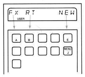
The **FX** menu label shows you that when you run PLY, the top left key on the calculator,  $\boxed{A}$ , is redefined to evaluate the polynomial f(x) at x.  $\boxed{B}$  (identified by the label **RT**) is redefined to compute the root, and  $\boxed{E}$  (identified by the label **NEW**) initializes the program to accept a new polynomial.
