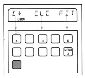
This menu will show you which key corresponds to which function in CFIT. Press J to recall this menu to the display at any time. This will not disturb the program in any way.
