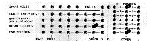
Note that, the program pins are inserted in a BIT POSITION hole when the ASCII/ISO codes, reproduced in Tables 1 and 2, give the corresponding bit as '1'.
