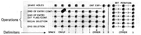
Note that, only one pin can be inserted in any column (i. e. delimiter may not initiate more than one operation).
