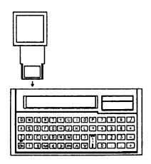
The adapter plugs into the HP-IL port at the back of the HP-71. First slide the cover off the port, then insert the adapter. Be sure the slot in the end of the interface is towards the bottom of the computer. Push in the adapter until it snaps into place.
