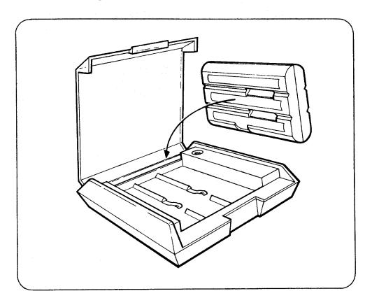
Put the battery pack into the holder with the battery pack contact strips down, so they rest on the contacts in the holder. Plug the recharger into the bottom of the holder and plug the other end into the wall socket.
