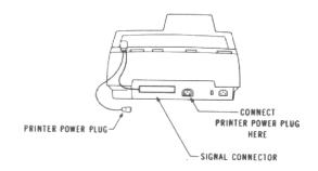
If the rear of the calculator has a receptacle which will accept the printer's power plug, connect the two. If the rear of the calculator does not have the receptacle connect the supplied adapter between the printer's power plug and a wall receptacle.
