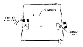
Turn the plastic wings from their stored position to the fully extended position. Notice the two circular holes that have appeared near the pivot point of the wings; they will fit over the thumbscrews on the calculator.
