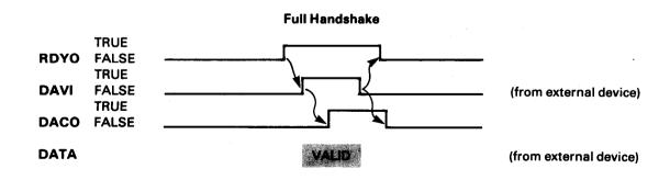
Logic System. The converter uses positive logic or negative logic for the data buses and for the handshake lines—each specified independently by control register R02-5,4.
