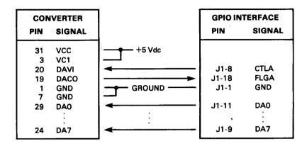
The next installation uses an 8-bit bidirectional data bus. The extra circuitry eliminates the need to modify the converter's control registers—the default values can be used. (The GPIO interface must have bit 0 of register 8 equal to 1—Output Enable A; other registers use their default values.)
