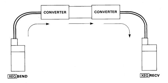
The following program is stored in each calculator. Execute RECV on the calculator that is to receive ALPHA data, and execute SEND on the calculator that is to send ALPHA data. Then enter a message at the sender followed by RIS.
