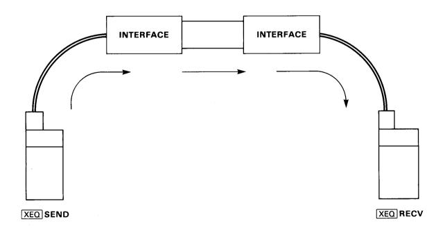
The following program is stored in each calculator. Execute "RECV" on the calculator that is to receive ALPHA data, and execute "SEND" on the calculator that is to send ALPHA data. Then enter a message at the sender followed by R/S.
