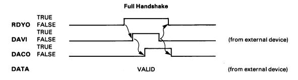
Logic System. The interface uses positive logic or negative logic for the data buses and for the handshake lines—each specified independently by control register R02-5,4.
