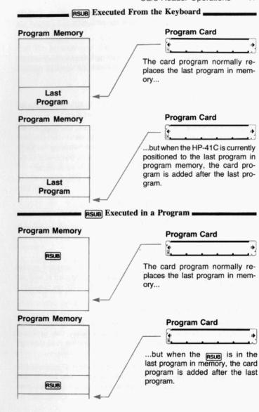
When you execute the **FISUB** function, either in a program or from the keyboard, the HP-41C prompts you for the card with
