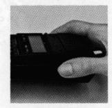
Pull the card reader straight back until the connector is free from port 4.
