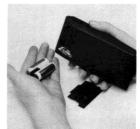
Place the new battery pack into the calculator. Your calculator will only turn on if the battery pack is inserted correctly.
