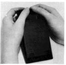
Turn calculator over and turn power on to assure proper battery installation. If the display does not light make sure the battery pack is correctly placed in calculator.
