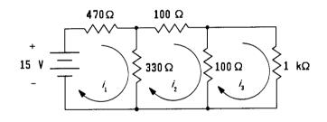
The following 3 equations are generated by summing the voltage drops around each loop.
