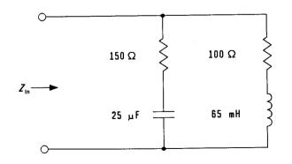
The elements in series are simply added to give the branch impedances  $Z_1 = 150 - i106.1033$  and  $Z_2 = 100 + i24.5044$ . The circuit is redrawn below.
