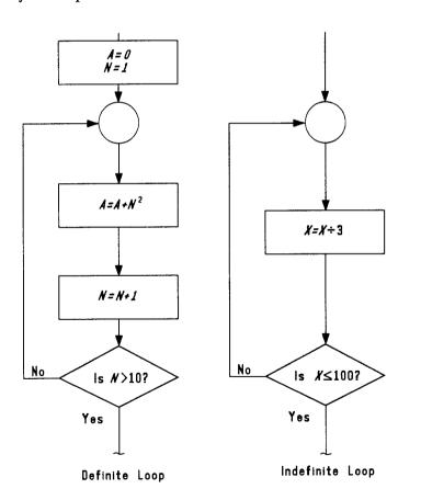
The definite loop illustrated in the figure will generate the sum of the squares of the integers 1 through 10. Notice that A is 0 initially, the loop counter N is 1 initially, and the loop counter is incremented by 1 with each pass through the loop. The definite loop is performed a *fixed* number of times (10 in this case). On the other hand, the indefinite loop repeats *indefinitely* until the desired condition  $(X \le 100)$  is met.
